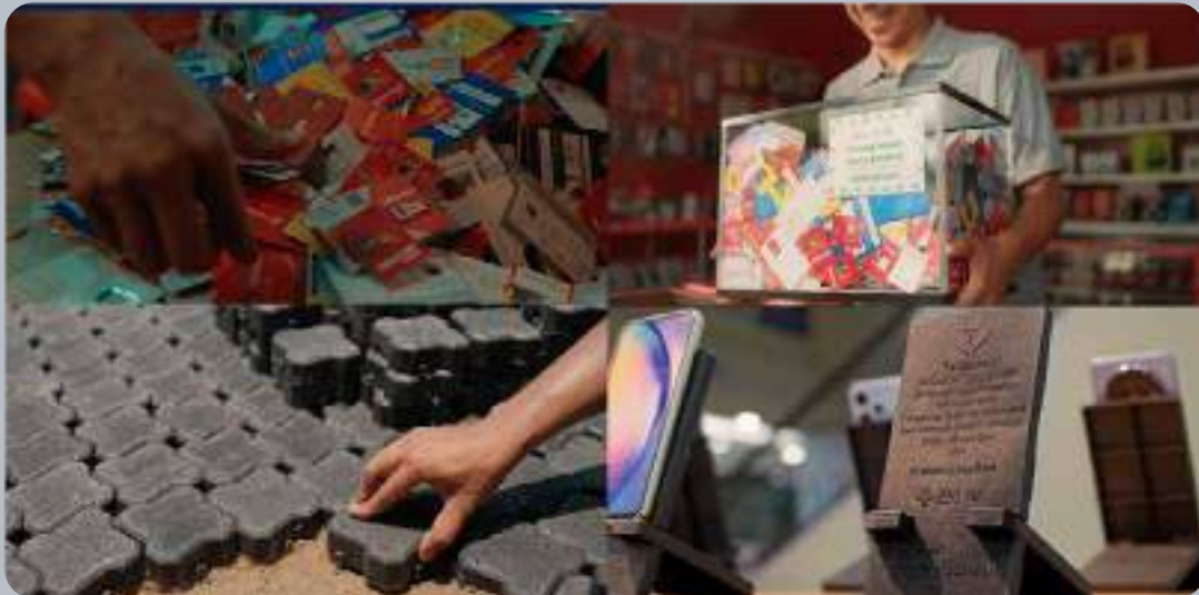
Figure 16. Paving block and phone holder from SIM card and its casing waste
